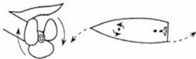
Right handed propeller – transverse thrust
