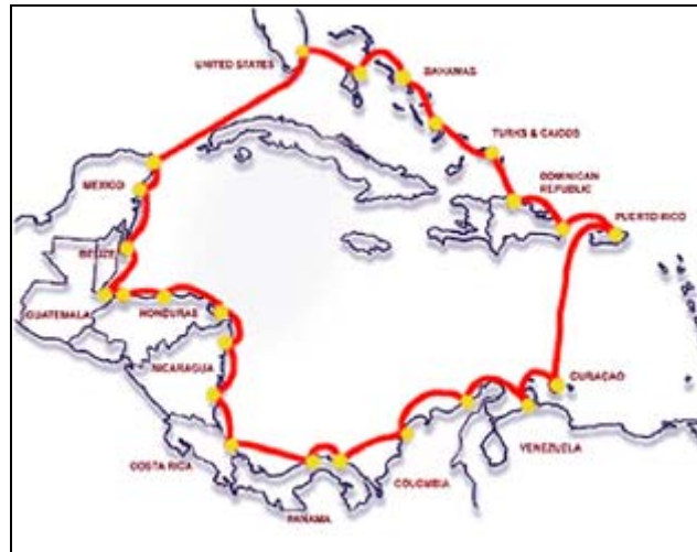
Figure 9. The Americas Region Caribbean Optical - Ring System (ARCOS) is an undersea fiber optic cable system that was developed to link the Caribbean region to the USA ( http://www.nearshore.cc/images/redundancyImage.jpg ).
